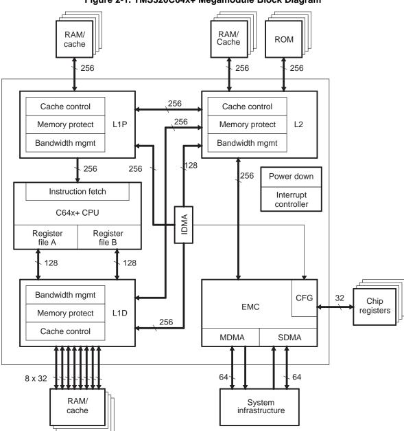
Figure 2-1. TMS320C64x+ Megamodule Block Diagram
